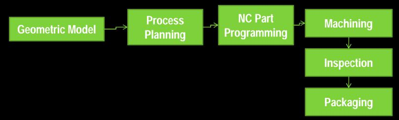
A Process of use of computers in planning, manufacturing, inspecting and controlling the manufacturing operation is called CAM
